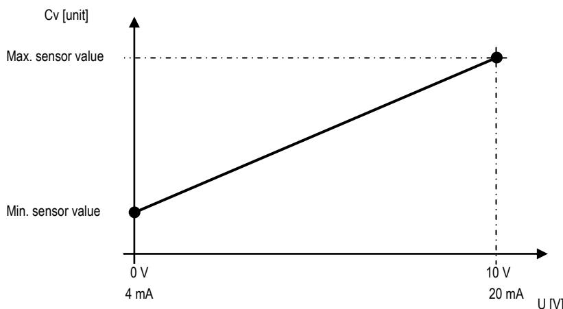
The specifications required for Min. sensor value and Max. sensor value can be found in the sensor data sheet.
