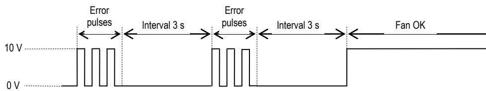
I/O 3 outputs a square-wave signal with levels 0 V (low) and 10 V (high)
