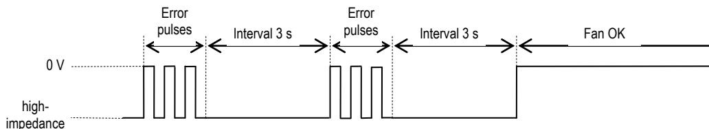
I/O 1 is designed as open collector output. A customer pull-up is required here.
