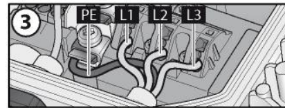
Fig. 2: Connecting the wires to terminals
