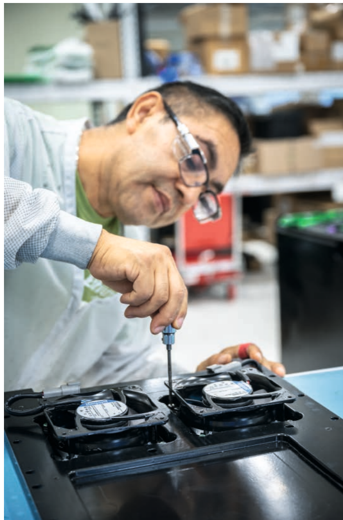
The robust and powerful compact fan is required for actively cooling the battery.
