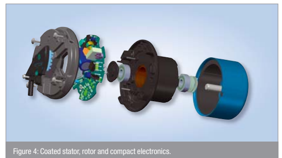
Figure 4: Coated stator, rotor and compact electronics.
